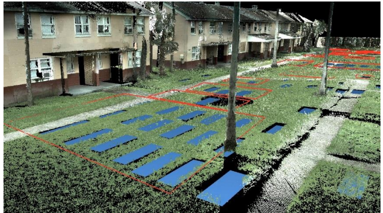
This image is a 3D laser scan of Robles Park Village showing grave-shaped objects beneath the ground in relation to buildings at the public housing complex. The single image is made from two data sources and aligns with historical maps of the former Zion Cemetery. [Cardno]
